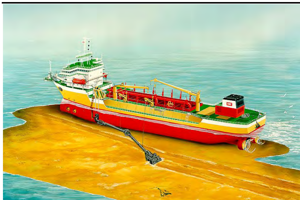
Figure 4.3 Illustration of a Trailing Suction Hopper Dredger
